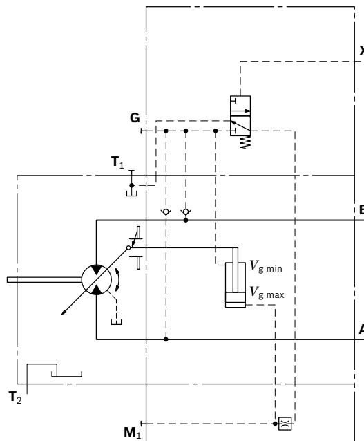
▼ Circuit diagram HZ7 (negative control) size 55 to 107
