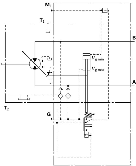
▼ Circuit diagram EP5, EP6 (negative control)
