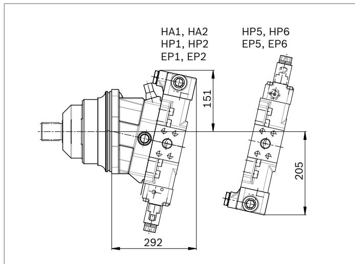
▼ Dimensions of sizes 160 and 200 (large flushing valve)
