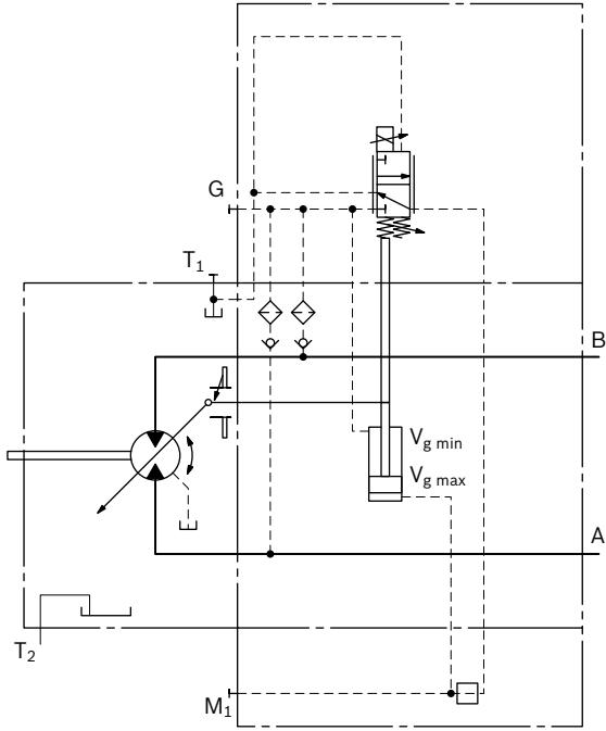
**EP5D1, EP6D1 Pressure control, fixed setting**
